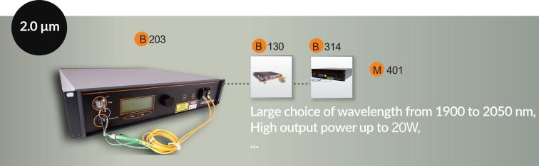
The CTFL-TERA series is a range of  $2\mu m$  Continuous Wave thulium fiber laser delivering up to 20W output power with random or linear polarization. The innovative all-in fiber designs offer a very good optical power stability with an excellent beam quality, M2<1.1 or M2<1.3 depending on the output power. Solutions are possible with a fixed operating center wavelength between 1900nm and 2050nm.
