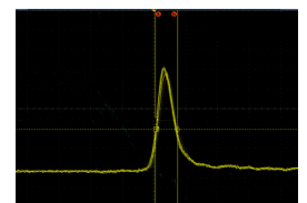
6 ns temporal profile @ 1064 nm with SLM option (1 GHz oscilloscope)
