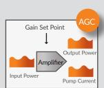
AGC (Automatic Gain Control) mode allows to control the amplifier at a fixed gain set point. The pump current is adjusted automatically to maintain the gain constant.
