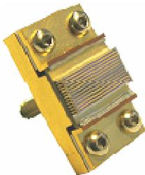
This stack "BS" type can be proposed with a variable number ('zz') of diode bars.
