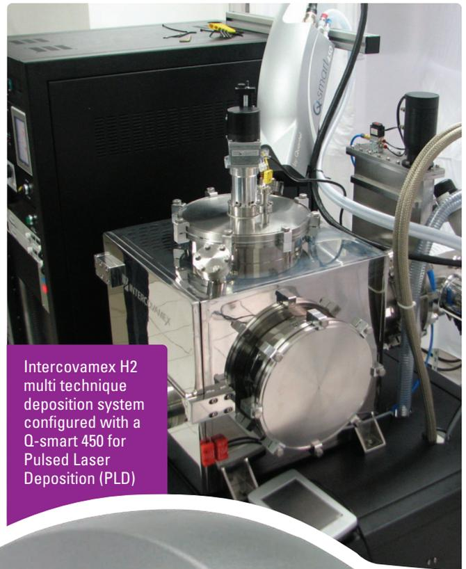
Intercovamex H2 multi technique deposition system configured with a Q-smart 450 for Pulsed Laser Deposition (PLD)
